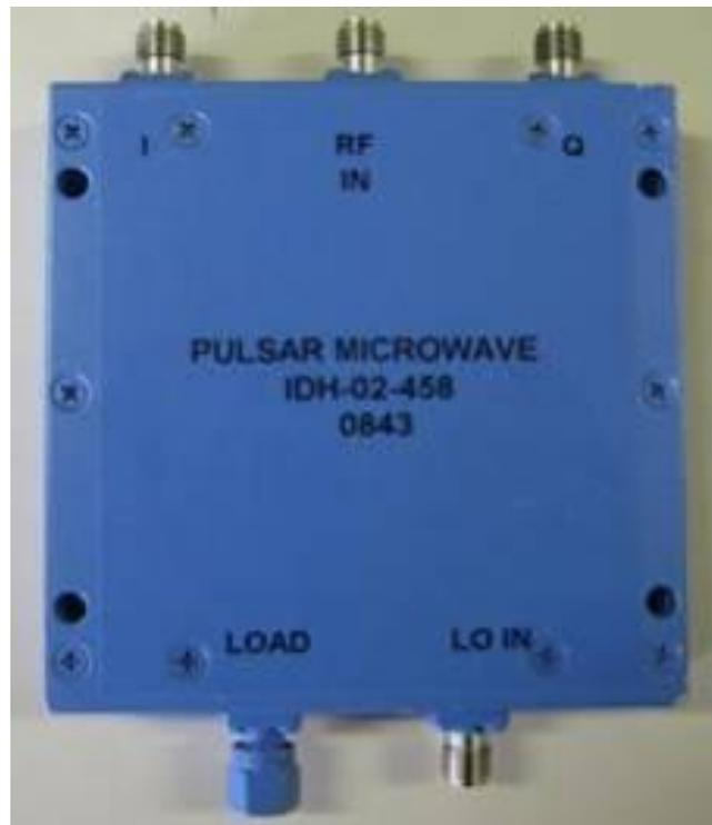
Fig. 3 Picture of the IQ demodulator.
