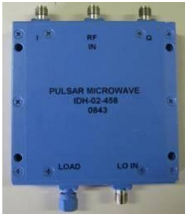
Fig. 3 Picture of the IQ demodulator.
